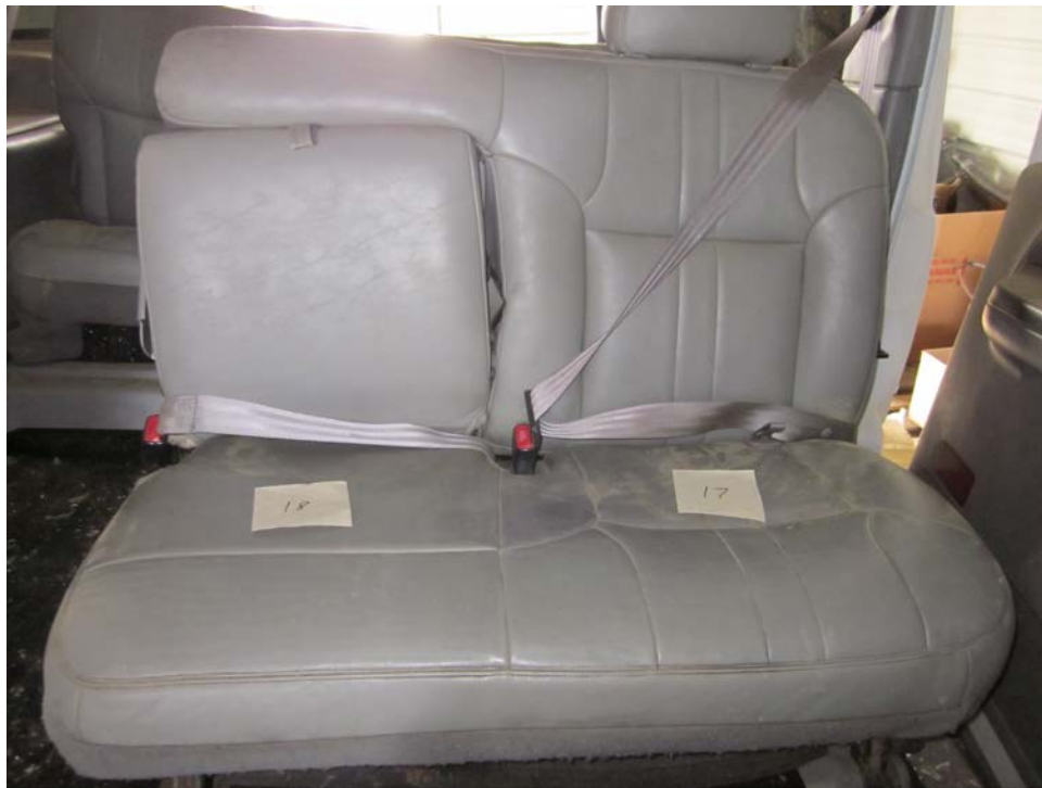
Figure 7. The rear OEM seats, which were deformed during the crash but remained structurally intact and attached to the floor. (Although the seat belts appear latched in this photograph, they were not found fastened after the crash.)
